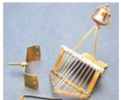
5 The brass cowcatcher and subframe to take the front 4 wheel bogie (LGB I think)
