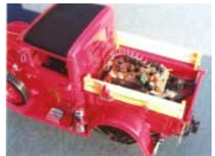
4 I wish I remembered where all the wires went! Rewire the batteries to the PCB via a new switch and connect up to the motor. The radio's 27mhz, with a 20-30' range.
